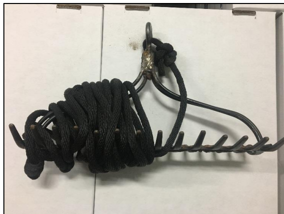
Figure 1: Double-headed, weighted garden rake, attached to a rope used to survey aquatic vegetation.
